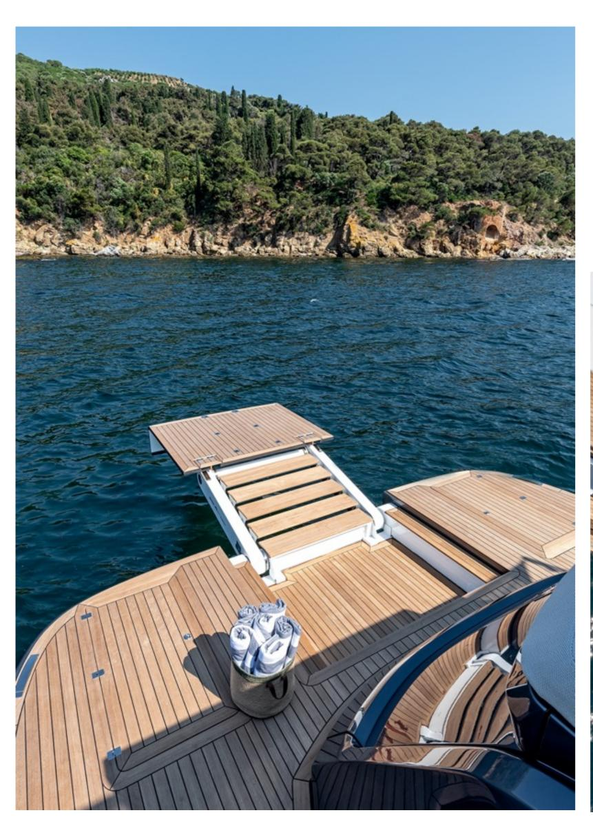
Alen 77 platform features a hydraulic mechanism that allows the entire stern area of the yacht to be lowered into the water, creating a spacious and stable beach club or water access platform. This functionality provides a seamless connection between the yacht and the water, enhancing the onboard experience.
